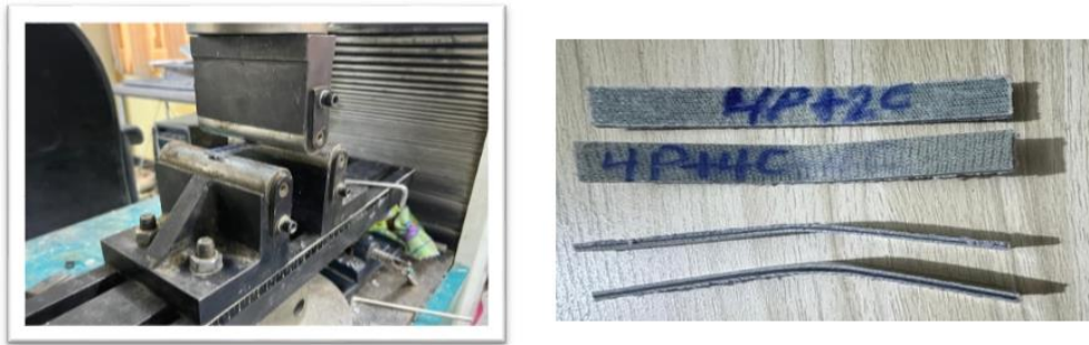
Figure 4. Bending test Machine and actual specimen: (a) Bending test machine (b) bending specimen
