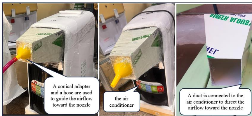
Figure 3. Air cooling system
